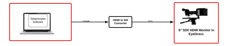
This is a simple solution to turn an EyeDirect into a Teleprompter. The process is the same as with a dedicated teleprompter except we are using a modified Eyedirect .
