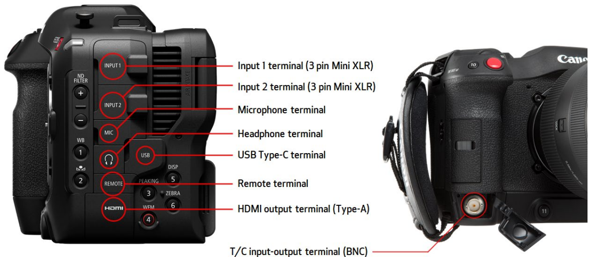
Figure 26 Most of the system interfaces are on the left hand side of the camera
